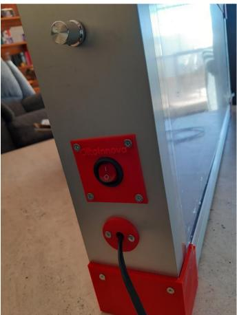
We have included a potentiometer for the control of the intensity of the leds. This is how we can adapt the lights for indoor and night races, in order to reduce glares that could be annoying for the public and the animals.
