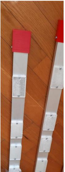
The reflector system consists of an aluminium bar that is 85 centimeters high, 4 centimeters wide and 2 centimeter deep. This aluminium bar is lightweight and handy. Every reflector is bolted and colocated at the exact high needed for a good infra-red laser reflection.
